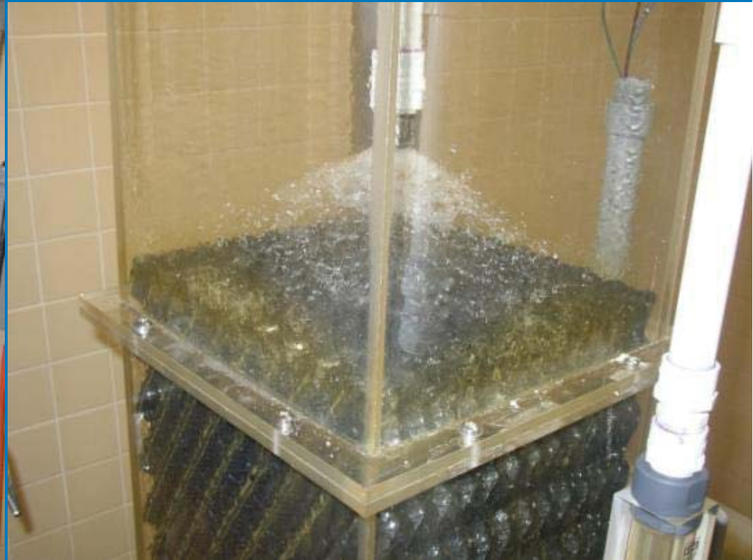
Water Distribution in Tower 2
